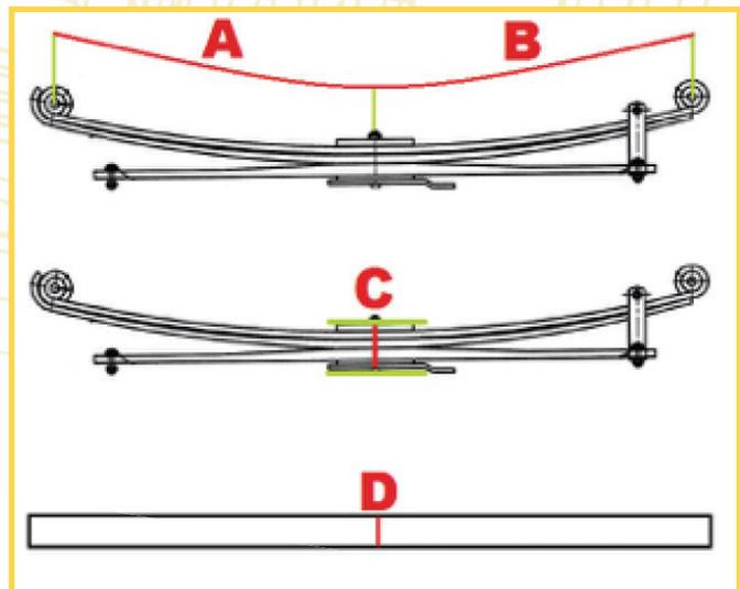
**Please note that measurements of width and thickness should be taken with a vernier calipers and length is most easily and accurately measured with a steel ruler as opposed to a measuring tape.**
